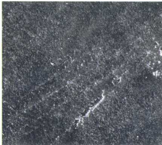
194 Differently polished surfaces of microfilled composites Left: Microfilled composite polished with medium-fine Super snap disk.
